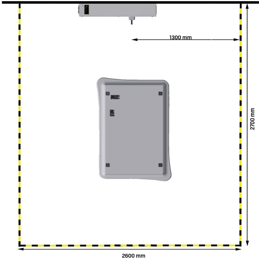
3.3. The floor around MiRCharge 24V must be marked to indicate the space that should be clear of obstacles and people when the robot is docking. This can for example be done with signal tape.
