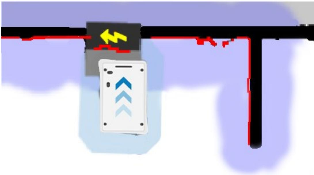
5.1. The red lines represent what the laser scanners see. The robot is correctly localized when they align with the black lines that represent walls.
